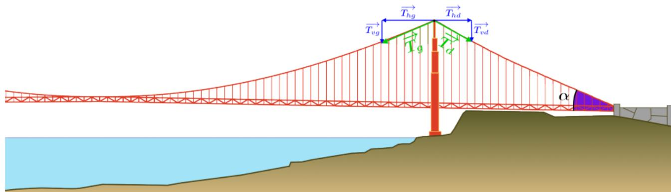
$$T_g = \frac{Mg}{2} \sqrt{\frac{L^2}{16h^2} + 1}, T_v = \frac{Mg}{2} \left( 1 + \frac{L \tan(\alpha)}{4h} \right) \text{ et } T_d = \frac{MgL}{8h \cos(\alpha)}$$
